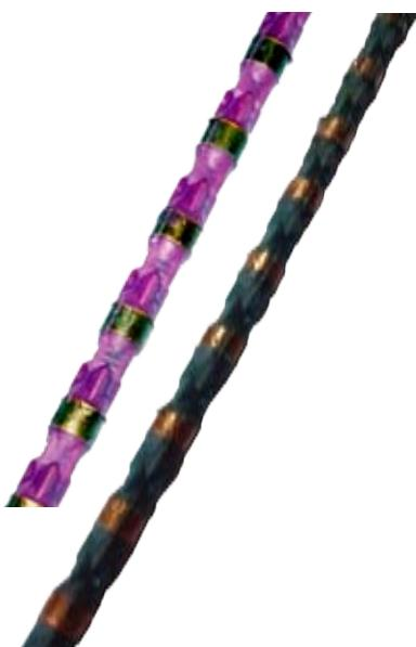
Sintered diamond wire for contour saw. The bead-Ø is 8,5mm or 11mm. The amount of the wire beads depends on cutting speed and machine power.
