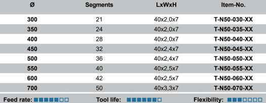
Application area: **Stationary systems**. Peripheral speed: **30 - 50 m/s**.
